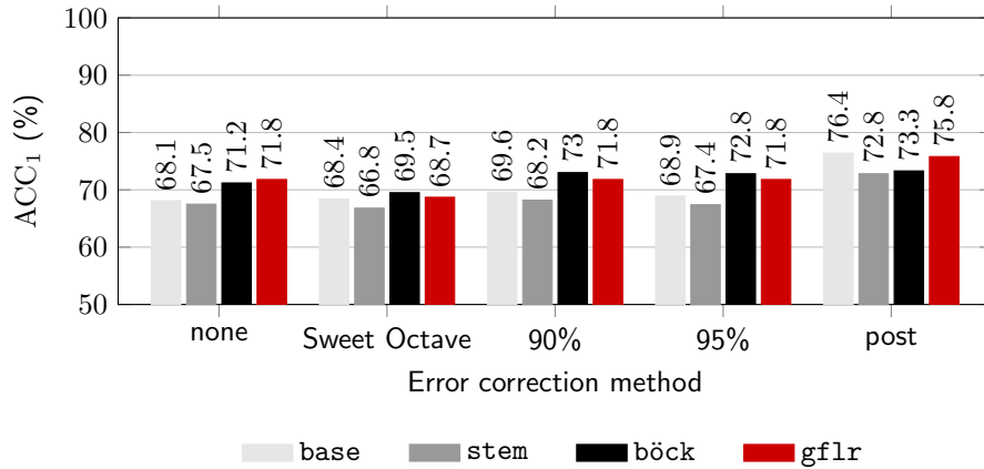
Figure 3.6.: ACC_1 for Combined using no error correction, constraint-based correction, and post correction for various tempo estimation algorithms.
