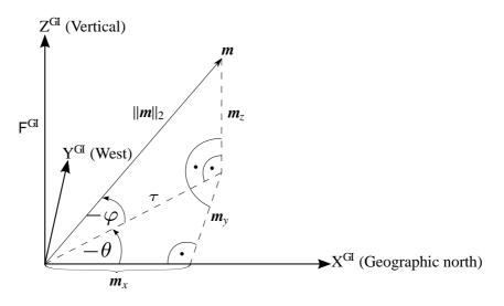
Figure A.3. Computation of the magnetic field vector m in the global inertial coordinate system  $F^{GI}$  using the inclination and declination angles.
