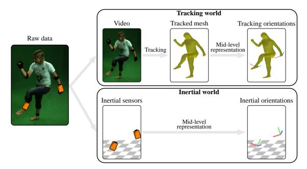
**Figure 7.1.** Raw data is recorded from video cameras and inertial sensors. In the tracking world, orientations are obtained by tracking. In the inertial world, orientations are derived from the sensor data.
