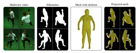
**Figure 7.6.** Overview of the silhouette-based tracking procedure [Rosenhahn *et al.*, 2007a]. Starting from multiview video, silhouettes are extracted by chroma keying. A skeleton-enhanced 3D model of the actor is then fit to the silhouettes based on optimization of joint angle parameters as well as the root orientation and translation.
