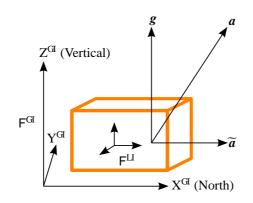
Figure A.4. The measured acceleration a is an overlay of the acceleration due to the motion  $\tilde{a}$  and the acceleration due to gravity g.
