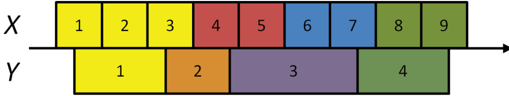
Figure 4.2: Illustration of our segmentation algorithm. The fixed-length input feature sequence X is transformed into the time-aware output feature sequence Y .
