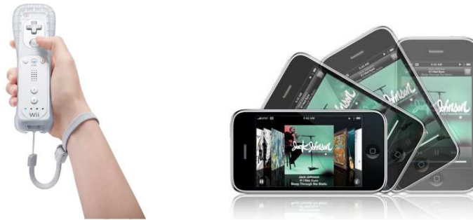
Figure 3.1. Inertial sensors are used in the Nintendo Wii Remote controller and the Apple iPhone 3 .
