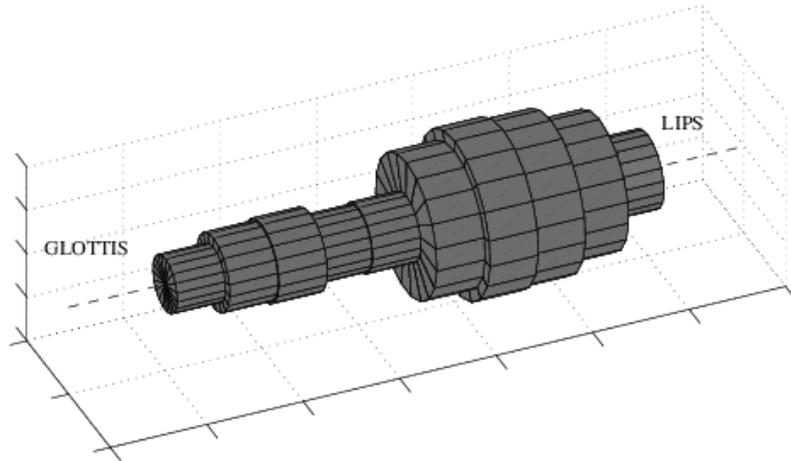
Figure 8: Illustration of the tube-model of speech production.
