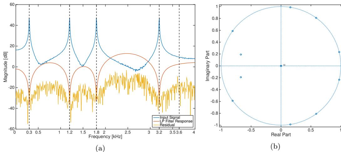
Figure 10: Linear prediction in the frequency- and  $z$ -domains. Depicted for a prediction order of 10. Figure (a) depicts the input signal, the filtered signal and the linear prediction filter response in the frequency domain. The dashed lines illustrate the exact positions of the roots of the filter. Figure (b) shows the roots of the linear prediction filter on the  $z$ -plane.
